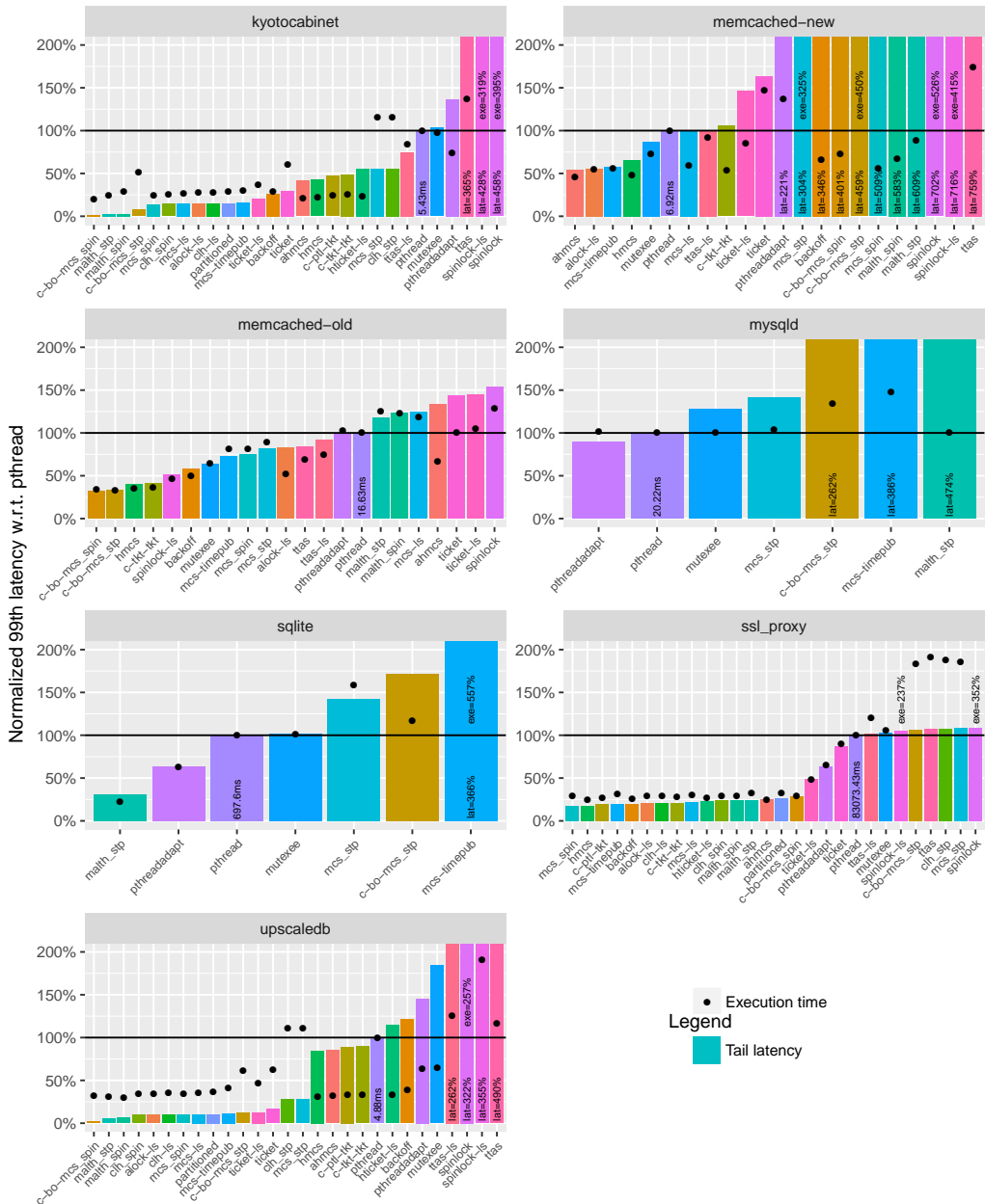
Fig. 29. For each server application, the bars represent the normalized 99th tail latency (w.r.t. Pthread) and the dots the execution time (lower is better) normalized (w.r.t. Pthread) of each lock algorithm (A-64 at max nodes).
